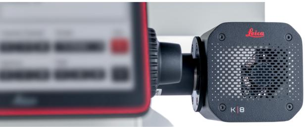
The K8 Scientific CMOS microscope camera offers a cutting-edge solution for the most challenging live-cell experiments. In an environment where sensitivity is everything, the K8 camera helps you capture more data from your sample, thanks to a 95% quantum efficiency (QE) back-thinned CMOS sensor.
