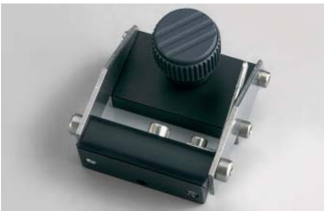
Special knife holder for sectioning specimens up to 20 mm high.
