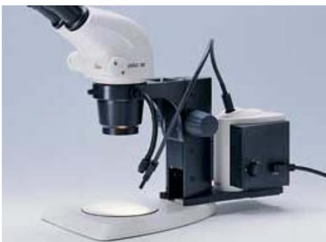
Leica L2 cold light source with arm for flexible light guide
