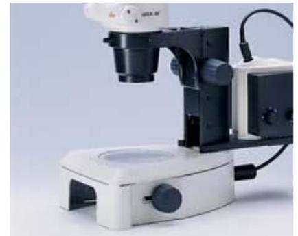
Transmitted light base and universal light guide for oblique transmitted illumination
