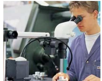
Leica S6 E with 60° viewing angle, tilted on swingarm stand
