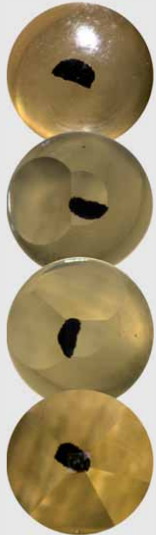
Steps to trimming a pyramid
